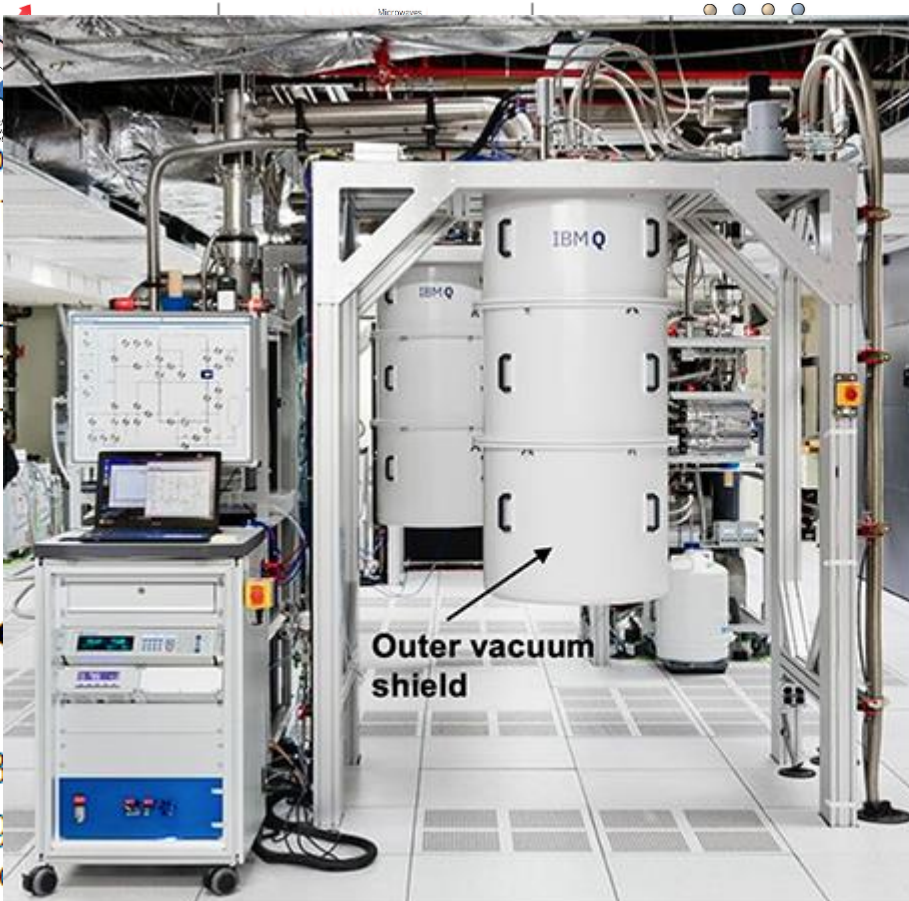
Dilution fridge setup: outside view
