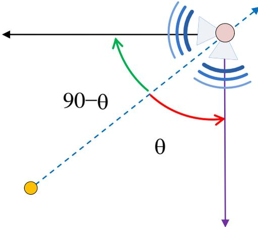
**Figure 10** Difference of the signal RSSI values received by two directional antennas with perpendicular orientations
