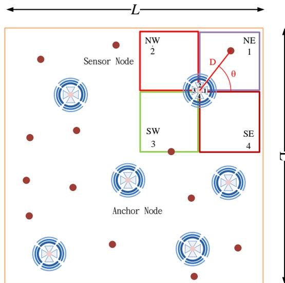
Figure 2 The setup for gathering and analyzing RSSI values
